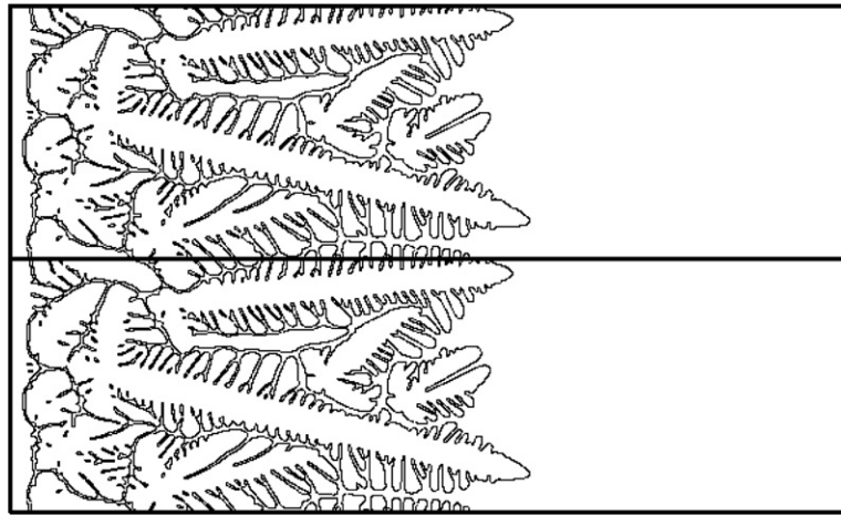
Fig. 23. Demonstration of sample problem domain with periodic boundary conditions applied at the top and bottom sides. The bottom half is the computational domain, the top half is just a copy of the solution from the bottom.
