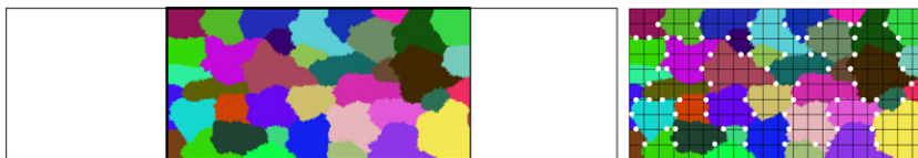
Fig. 3. (Left) Domain for computation (outer rectangle) and domain for performing averaging (inner rectangle). (Right) Schematic of the process for obtaining microstructure features.
